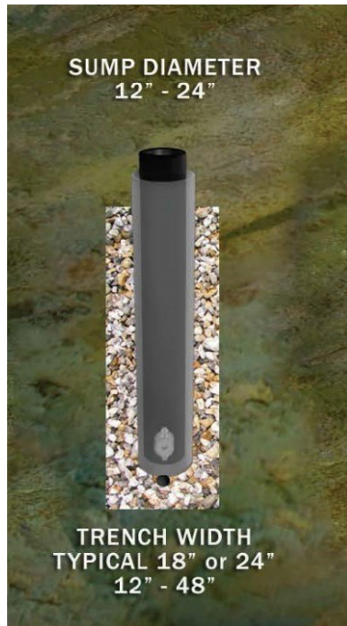
Figure 10-1: Typical Trench Design - Section
